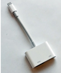
VZ 28: Apple Lightning Digital AV Adapter / Apple iPad/iPhone/iPod Videokabel Apple Lightning-Stecker HDMI-Buchse
